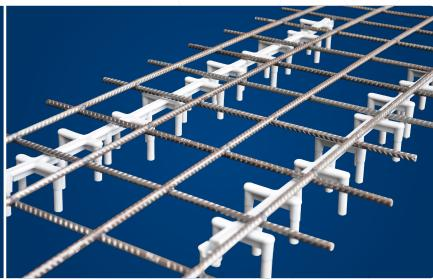
The 750mm long plastic Deck Rail is a continuous spacer which is strong and stable for formwork applications. The Deck Rail is designed with sets of vertical legs at approximately 75mm centres, allowing a free concrete flow. The legs have pointed tips on the base for minimal form contact. Deck rails have a clip connection system at each end to enable joining to any given length on site. Once connected the clip will not separate.
