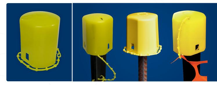
Novaplas manufactures UV Stabilised Bar Guards and safety caps that reduce the chance of cuts and abrasions from exposed reinforcing bars. Suitable for bar from 12mm to 36mm. Bar guards also fit over star pickets and have a connecting tie which attaches to the post. This tie prevents the cap falling off. Bar guards are not designed for high load vertical impacts.
