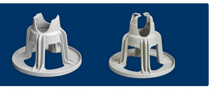
Our slab on ground bar chairs are light weight and stackable for ease of handling. These dual height reinforcement spacers are designed for ground floor slabs where support for steel is required without puncturing the polymer membrane. Manufactured from selected recycled plastics for superior performance. Supplied in coloured bags for easy size identification.
