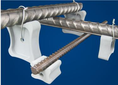
Novabone bar spacers have been designed specifically for heavy weight and large diameter reinforcing bars used in concrete beams for structures such as bridges.
