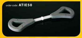
50 - 70mm Cavity is the standard medium duty Ni-Tie with each end over moulded with a resilient material. The resilience substantially reduces air and structure borne noises. Also reduces impact and vibration in masonry walls.
