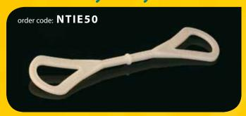
50mm Cavity Ties in Medium duty (white) to satisfy AS/NZ 2699-2000. Rounded ends to prevent injury and central hole to assist bond in mortar.
